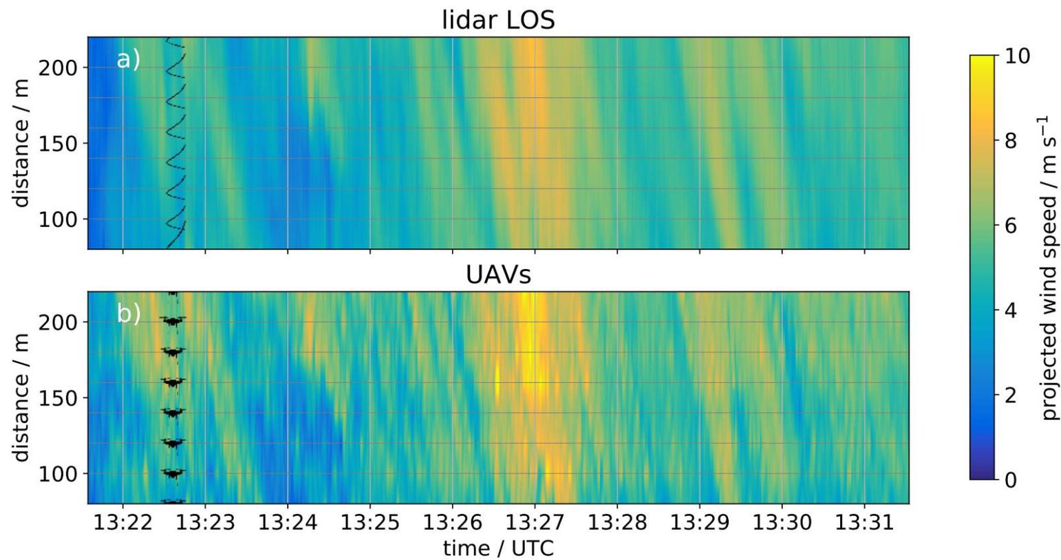
→ Flow structures detected by the lidar can be observed in UAV results
