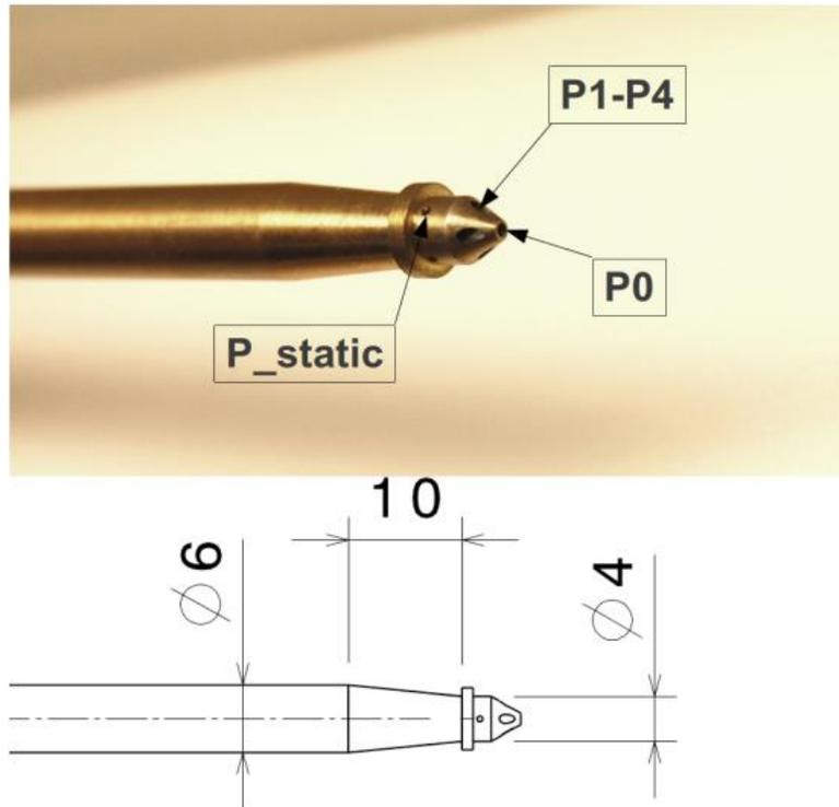
$$|\mathbf{v}_{\text{tas}}|^2 = 2c_p T_{\text{tot}} \left[ 1 - \left( \frac{p}{p+q} \right)^{\kappa} \right]$$
