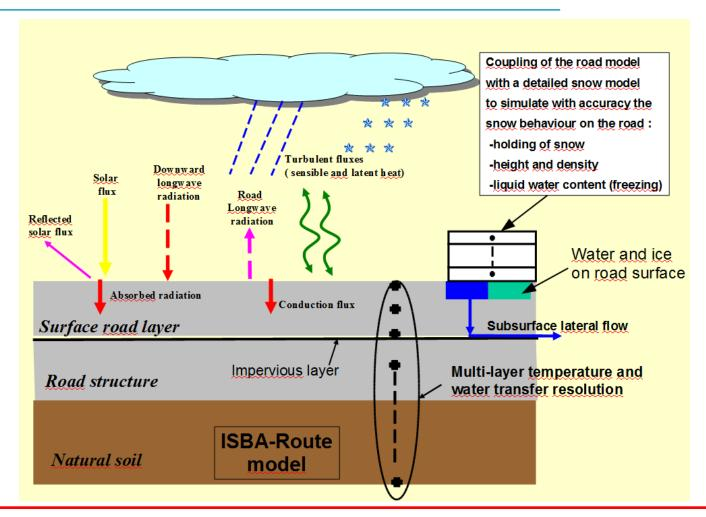
Outputs: road surface temperature, ice and water height on raod, snow height and type on the road....
