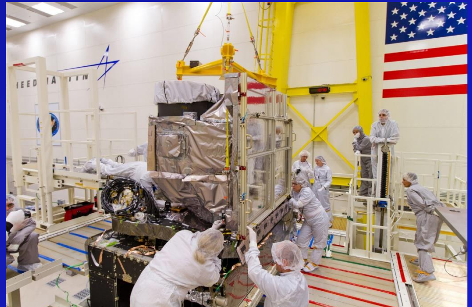
The Advanced Baseline Imager being installed on the GOES-R spacecraft
