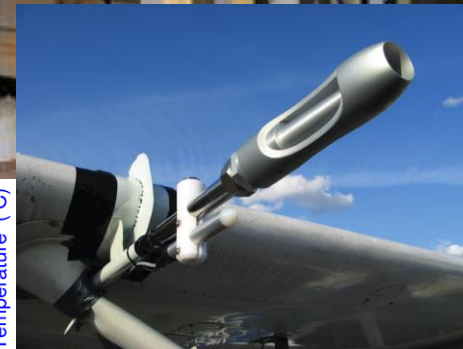
Fig. 1. Photographs of the inlet mounted on the right wing of the measurement aircraft.
